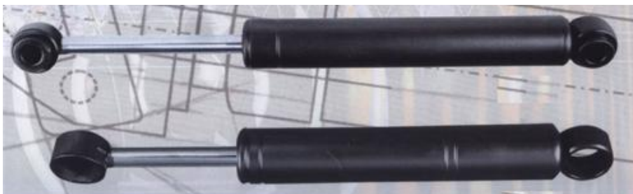
Figure 3.3: A hydraulic damper increases its resistance to motion in direct proportion to speed.
