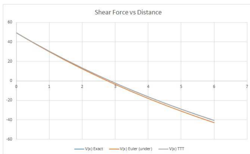
Figure 2.36: The following are h = 0.5 Euler and Three-Term-Taylor Method Approximations to the exact solution. The Three-Term-Taylor Method is almost indiscernable from the exact solution for this problem.
